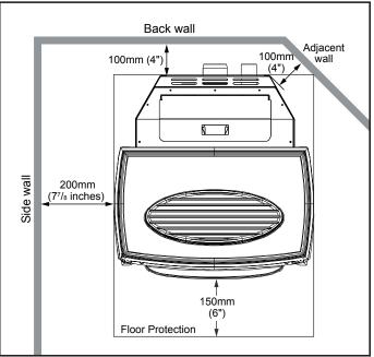
Figure 3: Minimum Clearances to Combustibles for Freestanding Windsor.
